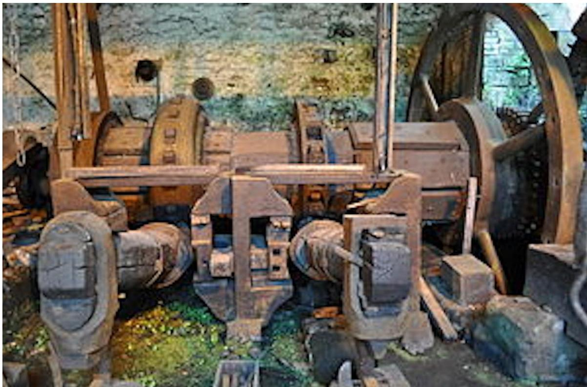
Note the cams on the axil of this double hammer machine, which tripped the two hammers closest to the camera. Not seen in this lower photograph are the two anvils under the hammers, but the single hammer machinery seen in the upper picture does show the anvil. The belt in the upper picture is driven by a water wheel.
